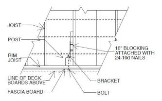
**Note:** if a single connector is used a 2x blocking cleat must be fitted against the bottom of the post along the joist or blocking to ensure post can with stand identical minimal code stipulated load from both directions.
